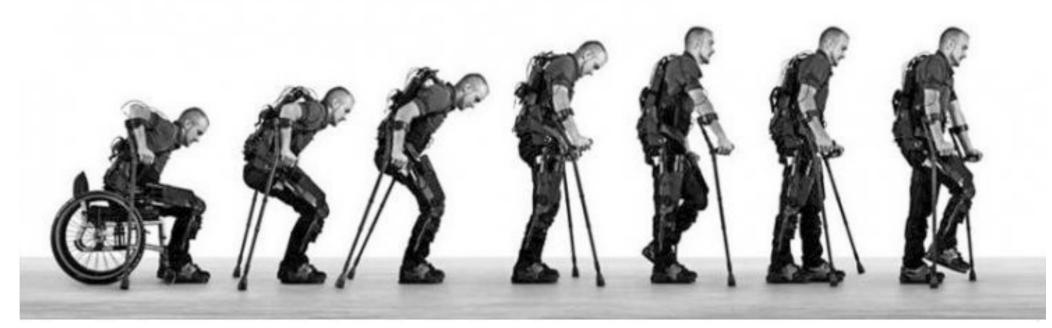
The Exoskeleton Sit to Stand. Image Courtesy of the No Barriers Foundation
